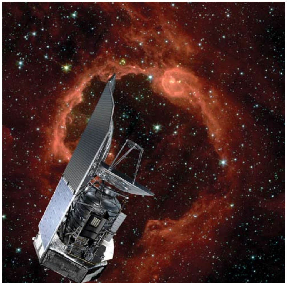
The Herschel Space Observatory has 3.5-meter primary mirror, allowing astronomers to see colder, darker celestial objects than ever before.
